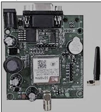
Fig. 5: GSM Modem
