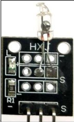
Fig. 4: Tilt Sensor
