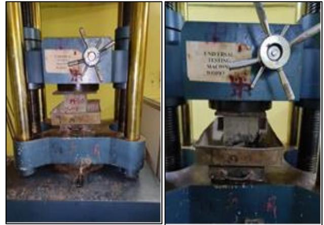
Fig. 4.1: Compressive strength Test on UTM before & after failure
