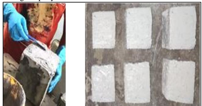
Fig. 5.2: Repairing the cracked concrete cubes with epoxy
