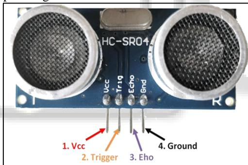
Fig. 5: Ultrasonic Sensor
