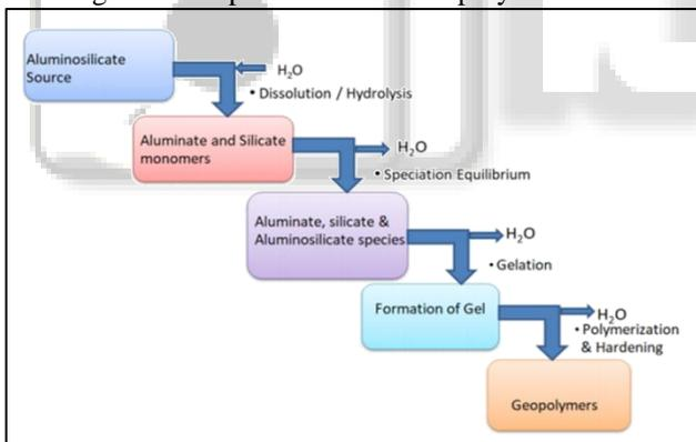
Fig. 1: Conceptual model of Geo-Polymerisation.
