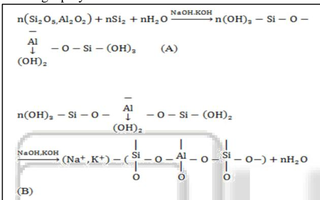
Fig. 1: Conceptual model of Geopolymerization
