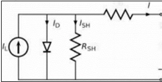
Fig. 2: Equivalent Circuit of Photovoltaic System
