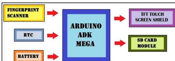
Fig. 4: Block Diagram of the Portable Attendance System
