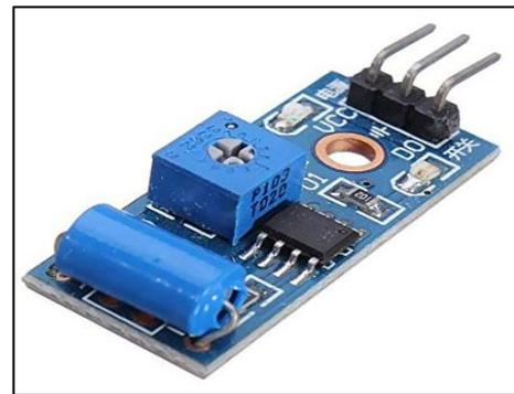
Fig. 3: Vibration Sensor
