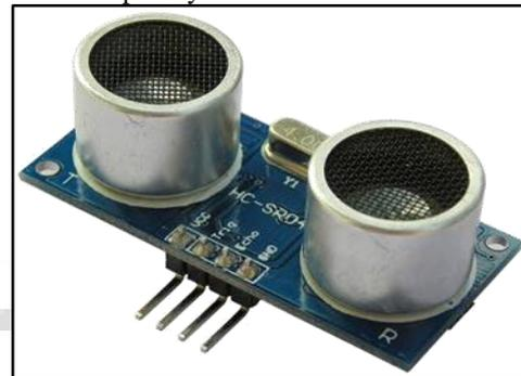
Fig. 4: Ultrasonic Sensor
