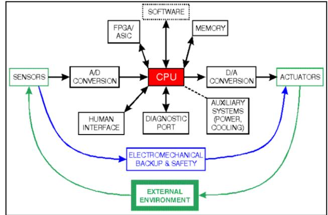
Fig. 8: Block Diagram of a Typical Embedded System
