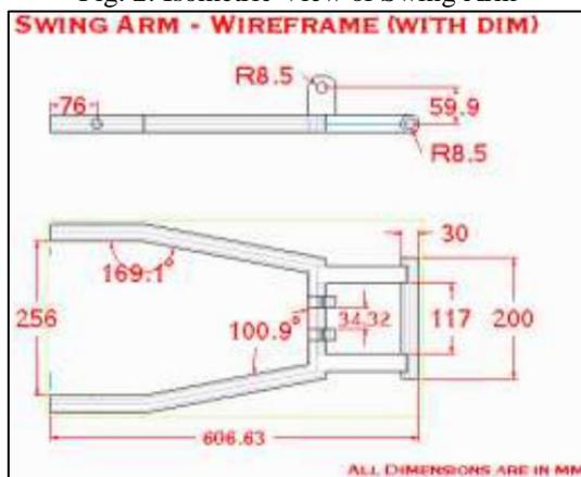
Fig. 3: Swing Arm with Dimensions
