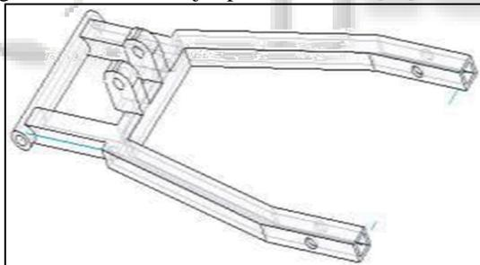
Fig. 2: Isometric View of Swing Arm
