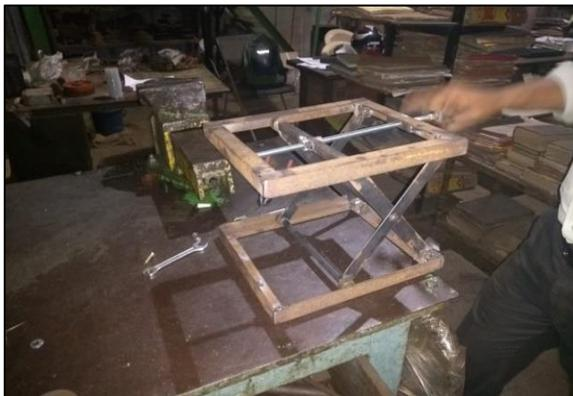
Fig.1: Lead Screw Lift Table
