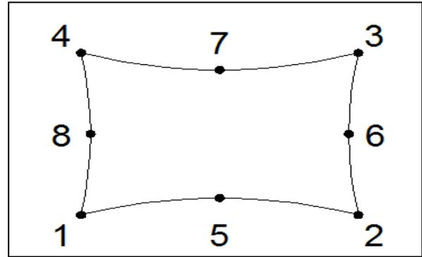
Fig. 2: Isoperimetric quadratic shell element
