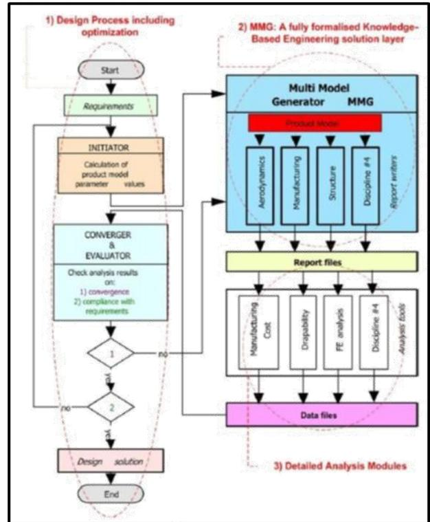
Fig. 8: Design Engineering Engine DDE methodology [Laan,V.D, et al., 2006].
