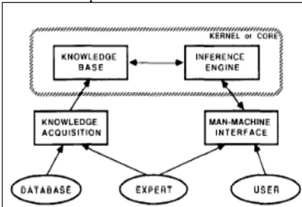
Fig. 2: Components and interactions of a typical knowledge-based system [Gilmore, M.L., 1989]
