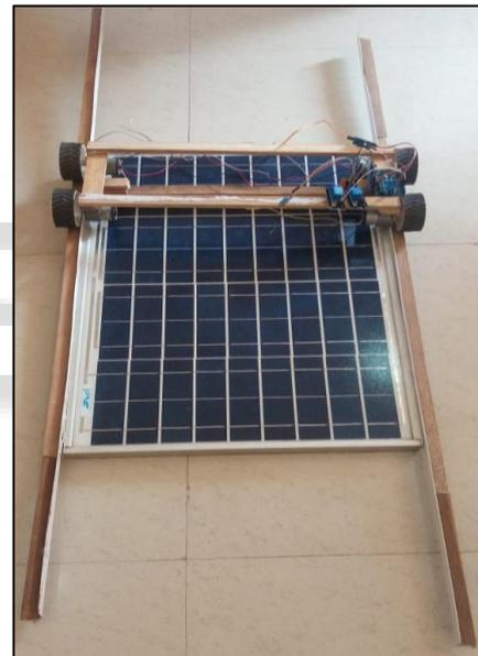
Fig. 9: Cleaning System for Single Panel
