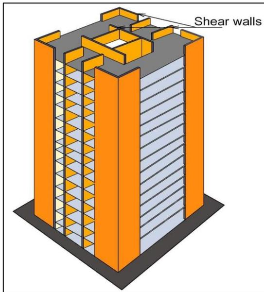
Fig. 1: Building with Shear Wall
