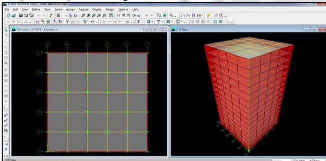
Model 2: Building with Structural Wall along Perimeter of RC Frame
