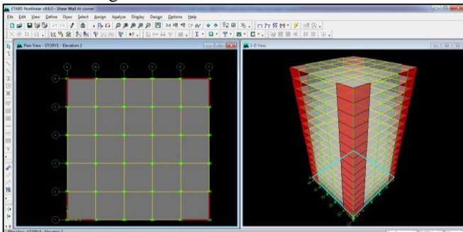
Model 1: Building with Shear Walls of RC Frame
