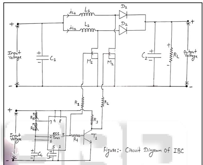
Fig. 1: Circuit Diagram of IBC
