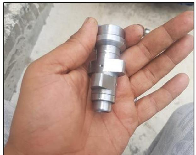
Fig. 2: Cam Shaft after Modification
