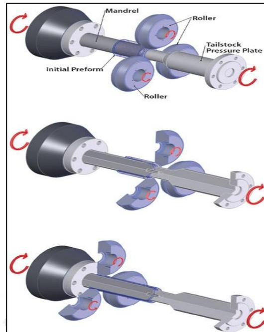
Fig. 1: Tube spinning by three roller spinning head
