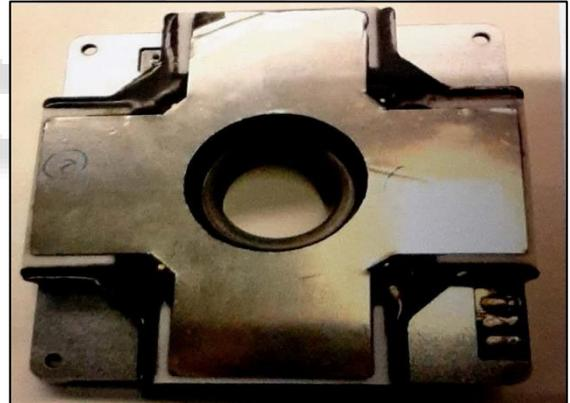
Fig. 9: Final product (4 roller spinning head)
