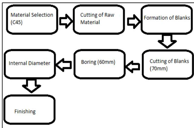
Fig. 7: Process sheet for fabrication of roller
