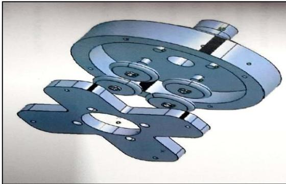
Fig. 6: Exploded view of four roller spinning head
