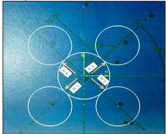
Fig. 4: Schematic diagram of radial spinning force exerted on mandrel with uniformly distributed rollers
