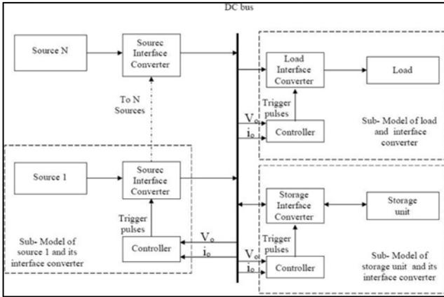
Fig. 2: Simulation model of hybrid renewable nanogrid.
