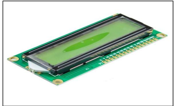
Fig. 3.8: LCD Display
