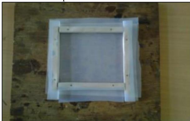
Fig. 1: Mould used for fabrication of composite
