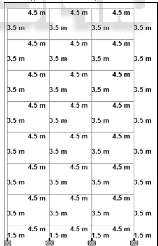
Fig. 2: Elevation of building frame model
