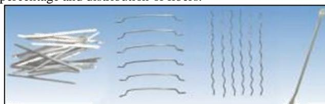
Fig. 1: Steel Fiber (a) Straight (b) End-hooked
