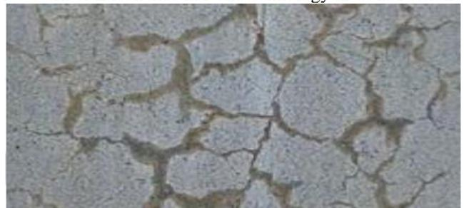
Fig. 2: ASR crack pattern for Nano Silica
