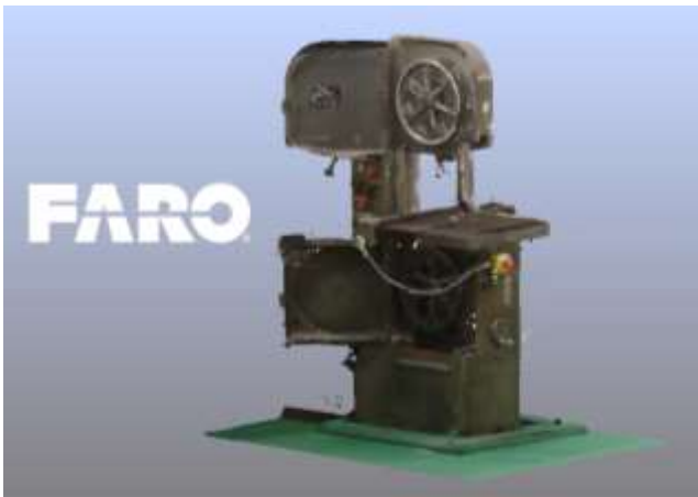
Fig. 2.0: 3D interactive scan of Equipment using Faro Laser scanner
