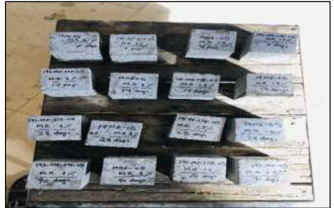
Fig. 2: Casted Concrete Cubes
