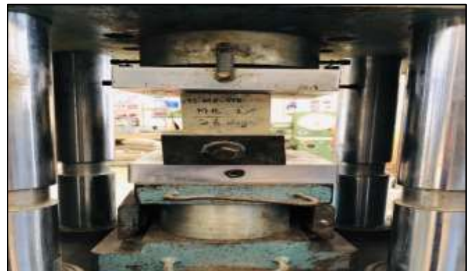
Fig. 4: Test Setup of compressive strength of concrete
