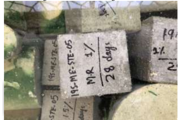
Fig. 3: curing of specimen
