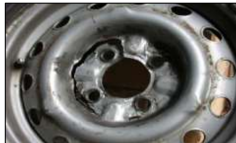
Fig. 1: Crack near the hub hole
