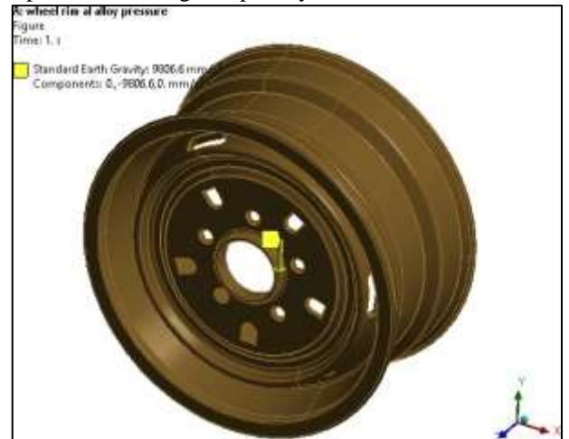
Boundary conditions for baseline wheel rim model
