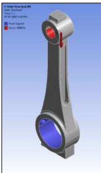
Static Structural Boundary Conditions and loading conditions
