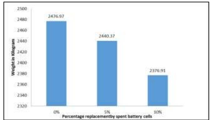
Fig. 2 Bar graph showing self-weight of concrete
