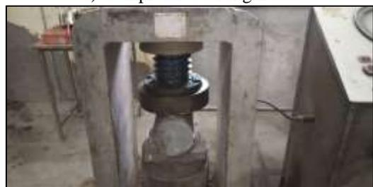
b) Split tensile strength test
