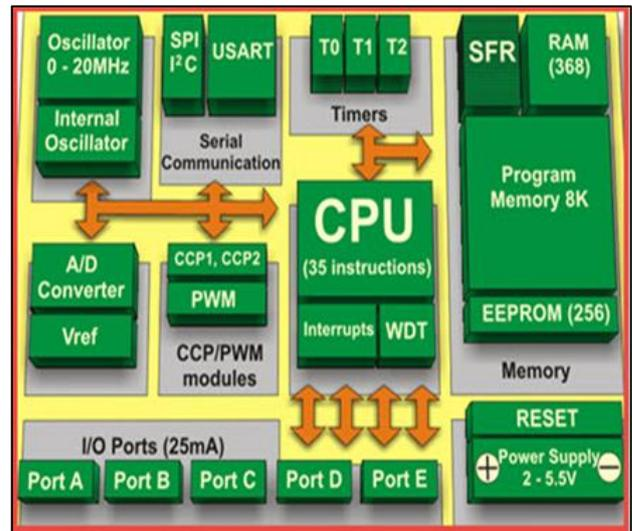
Fig. 1.3: Architecture of PIC16F877A
