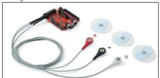
Fig. 2: ECG sensor
