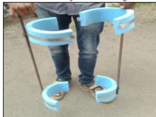
Fig. 3: Bolt and cushions of the leg mechanism
