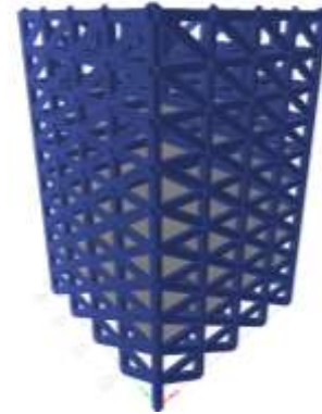
Fig. 1: Elevation of infill frame Model with Strut
