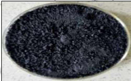
Fig. 3: Activated carbon produced using Sulphuric Acid
