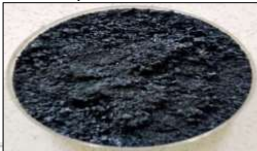
Fig. 2: Activated carbon produced using Phosphoric Acids
