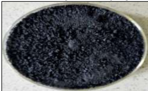
Fig. 4: Activated carbon produced using Zinc Chloride
