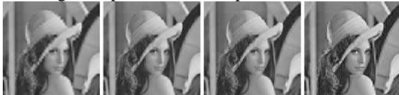
Fig 6 Compression of Lena using CB11 Approximate DCT method and Bit-level Exact Computing; (a) RC = 4, (b) RC = 10, (c) RC = 16,
