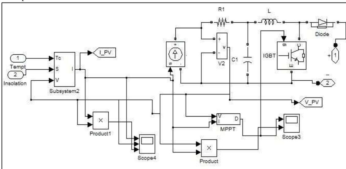
Fig. 11: Simulink model for Solar PV cell
