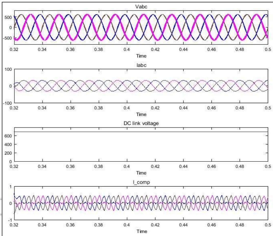
Fig. 14: Source voltage ( $v_{abc}$ ), compensated source current ( $I_{abc}$ ), dc link voltage ( $V_{dc}$ ) and compensation current ( $I_{comp}$ ) in steady state with SAPF and insolation  $1000W/m^2$
