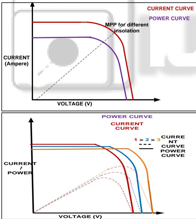
Fig. 2: Solar I-V and P-V curve (a) with different temperature insolation and (b) MPP for different Insolation
