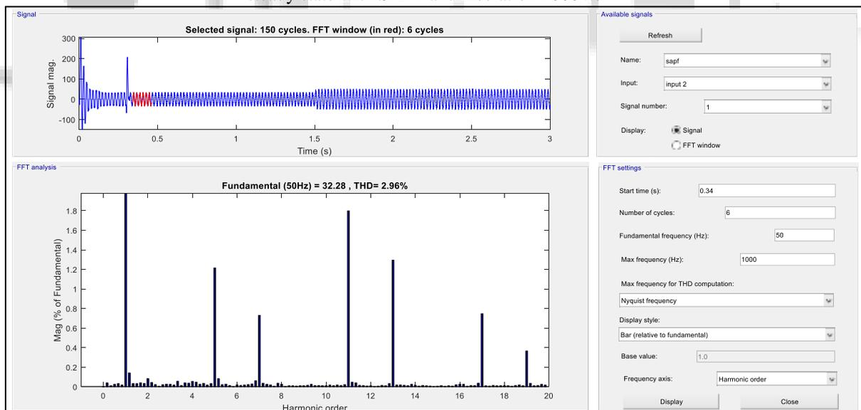
Fig.15: Frequency spectrum of compensated source current insolation  $1000W/m^2$
