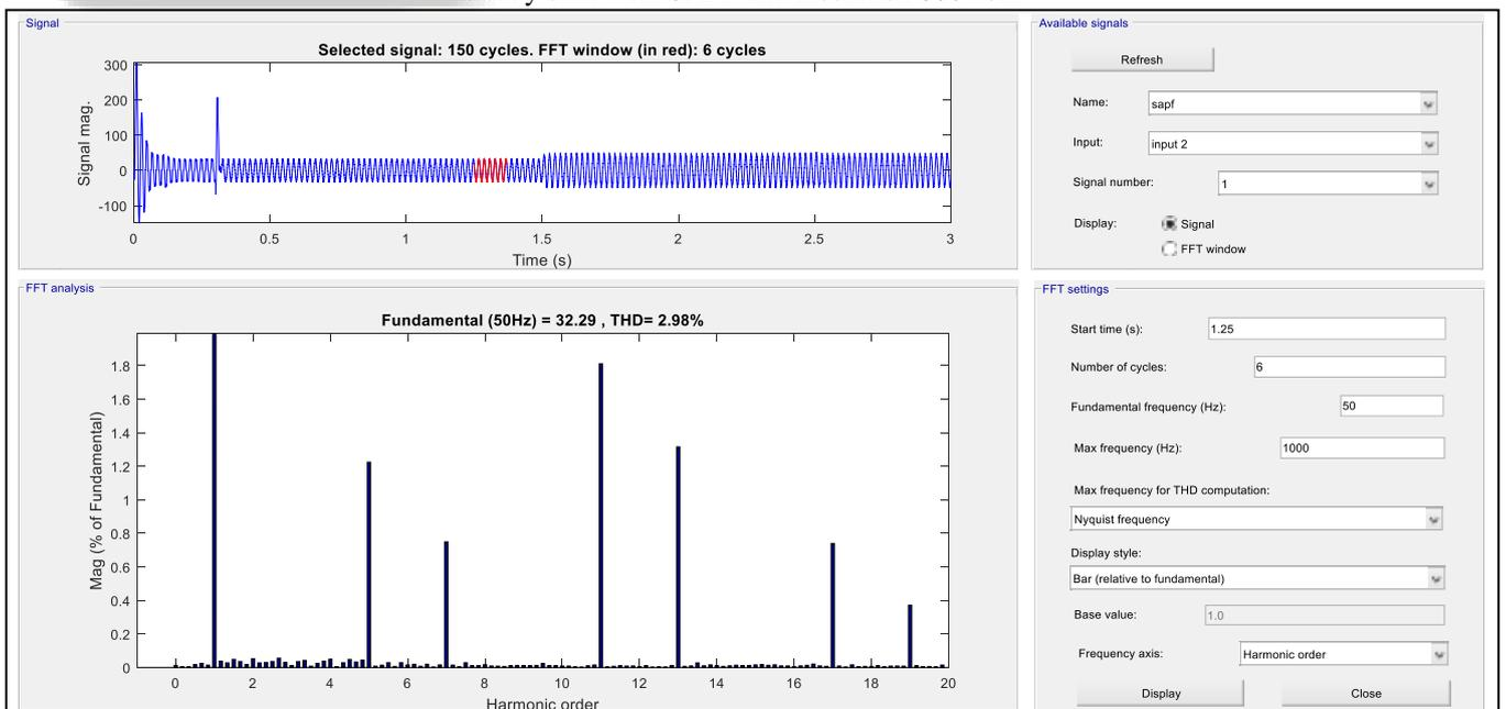
Fig. 17: Frequency spectrum of compensated source current insolation  $800W/m^2$
