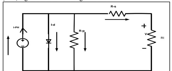
Fig. 4: Equivalent circuit of photo-voltaic cell
