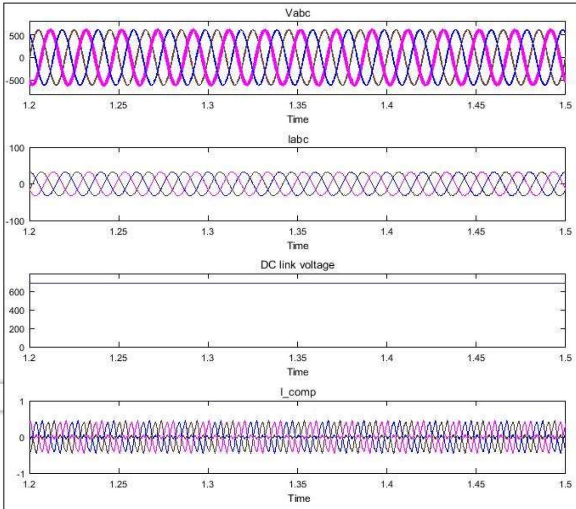
Fig. 16: Source voltage ( $v_{abc}$ ), compensated source current ( $I_{abc}$ ), dc link voltage ( $V_{dc}$ ) and compensation current ( $I_{comp}$ ) in steady state with SAPF and insolation  $800W/m^2$
