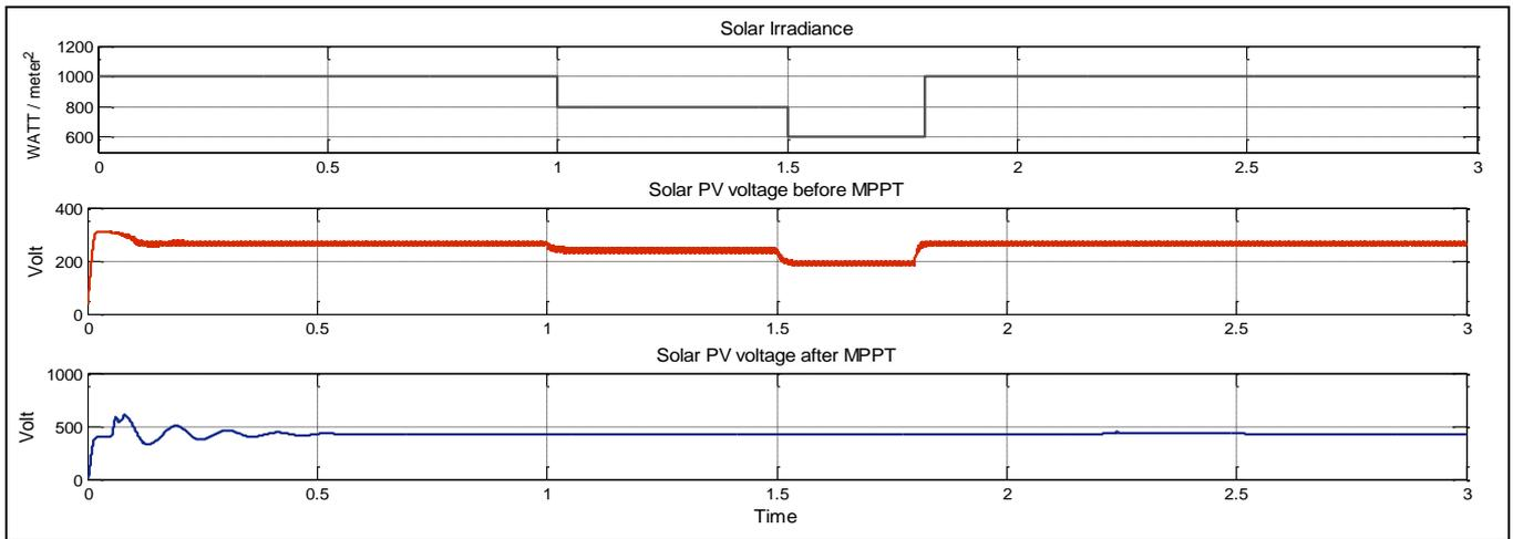
Fig. 12: Effect of solar Irradinance on the PV cell voltage before and after MPPT
