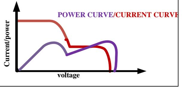
Fig. 3: (a) Operation of solar P-V under partial shading (b) P-V graph under same partial shading criteria
