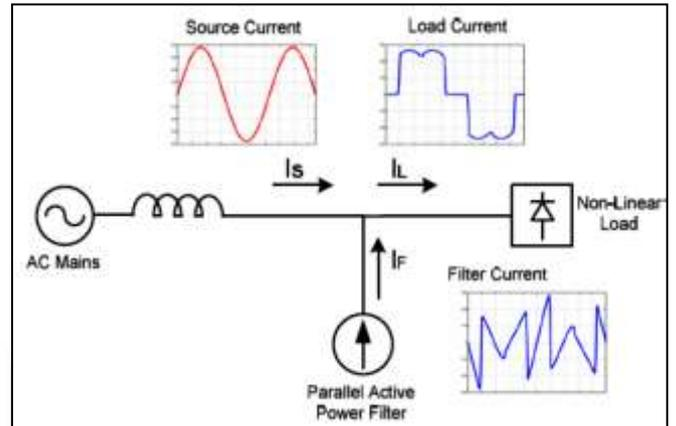
Fig. 6: Main Principle of Active Filtering
