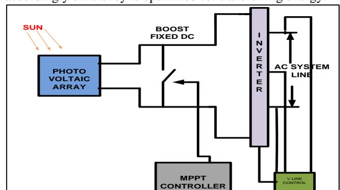
Fig. 1: Maximum power point tracker system
