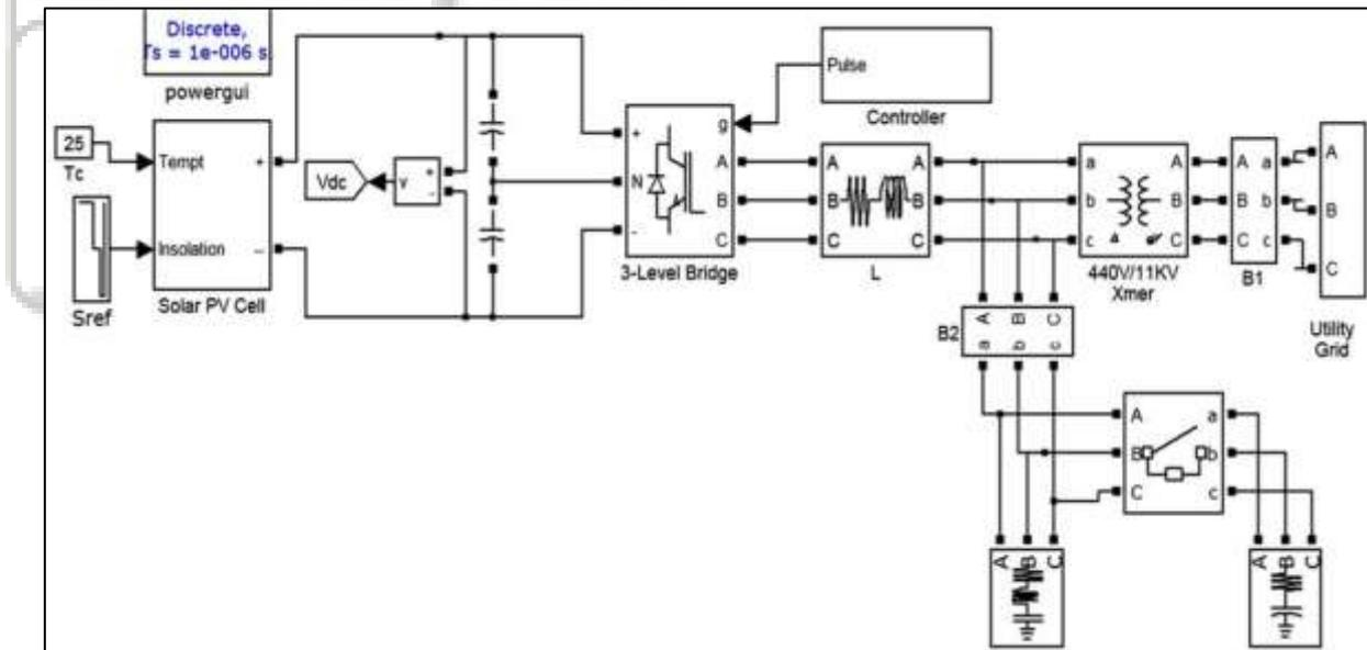
Fig 8: Simulink model of Grid connected Solar PV system
