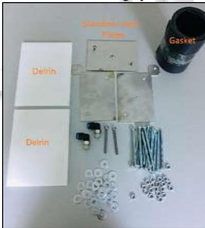
Fig. 1: Components of dry cell.
