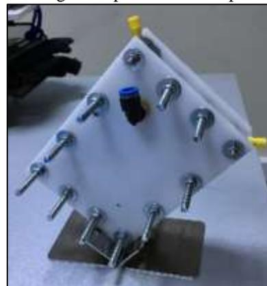
Fig. 4: Manufactured dry cell
