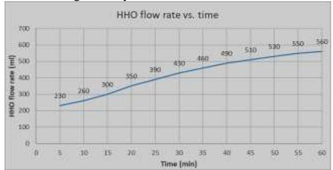
Fig. 6: Generated HHO gas in terms of time at constant voltage
