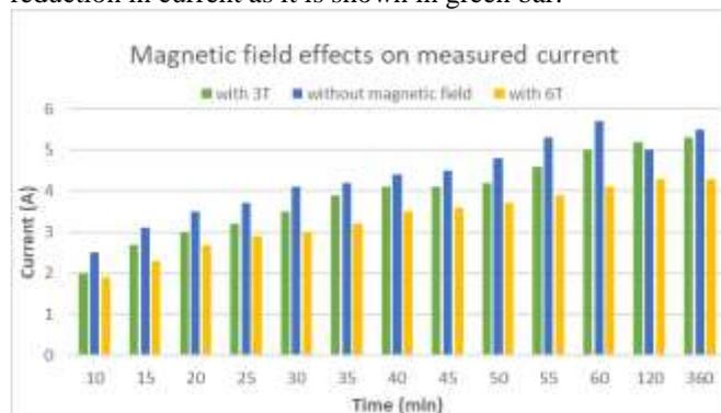
Fig. 7: Changing current with or without magnetic field at constant voltage
