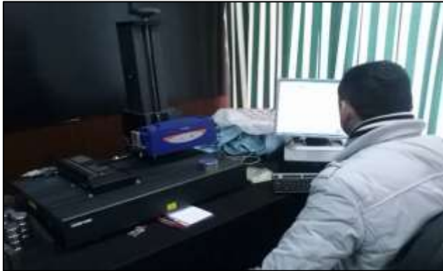
Fig. 4: The measuring device for measuring the roughness of processed surface TALYSURF-INTRA
