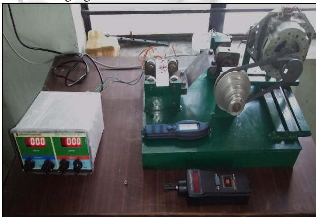
Fig. 3.1: Experimental set up of Transverse Vibration Test Rig.
