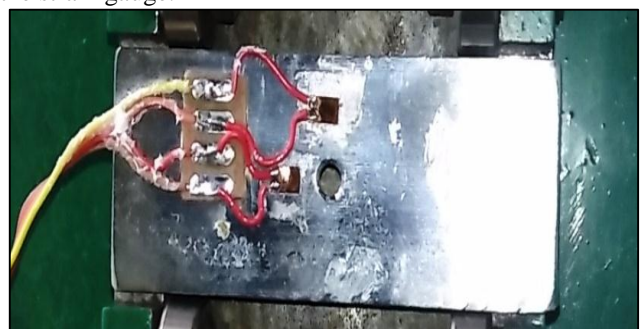
Fig. 3.3: Image of Mounting of Strain Gauge
