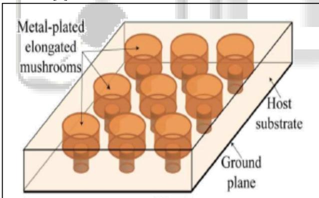
Fig. 4: Elongated Mushroom Electromagnetic Band Gap (EM-EBG) structure
