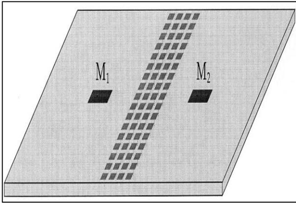
Fig. 3: Microstrip antennas separated by the mushroom-like EBG structure (CM-EBG)
