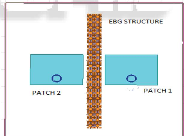
Fig. 2: EBG structured 2x1 microstrip antenna.
