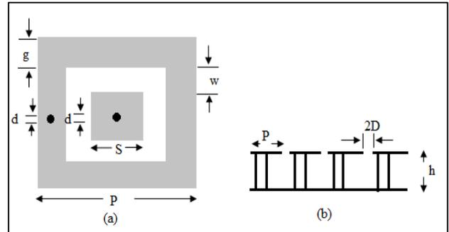
Fig. 1: Two via Slot type Electromagnetic Band Gap (TVS-EBG) structure (a) top view (b) side view.
