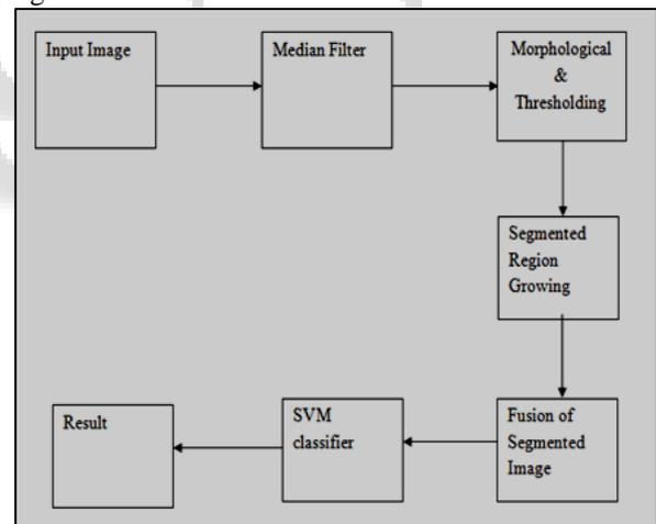
Fig. 1: Block Diagram of the Brain tumor Detection
