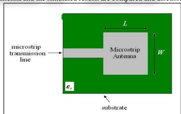
Fig. 2: rectangular patch antenna
