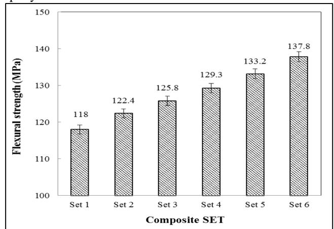
Fig. 3: Flexural strength of epoxy/short sisal fiber composites
