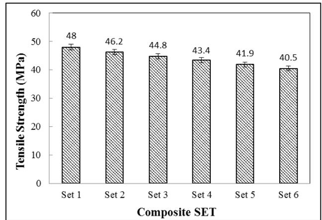
Fig. 1: Tensile strength of epoxy/short sisal fiber composites
