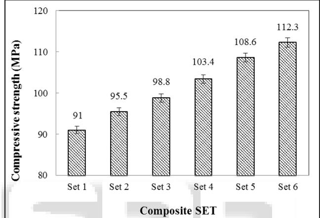
Fig. 2: Compressive strength of epoxy/short sisal fiber composites
