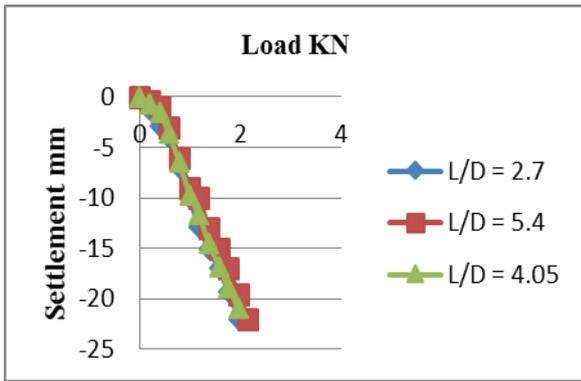
Fig. 6: comparison of granular pile formed using aggregates with varied L/D ratio
