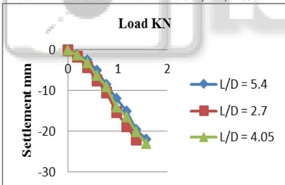
Fig. 8: comparison of granular pile formed using tile waste with varied L/D ratio
