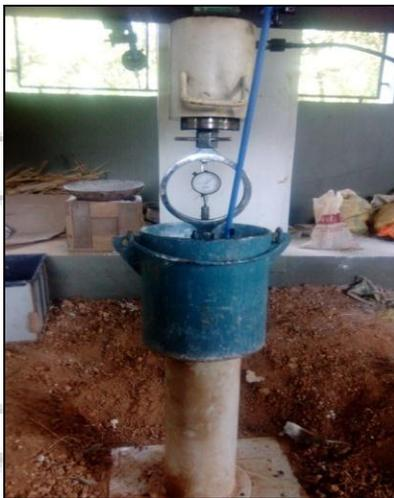
Fig. 1: Test setup for vertical loading
