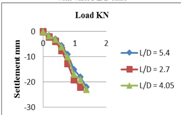
Fig. 9: comparison of granular pile formed using brick waste with varied L/D ratio
