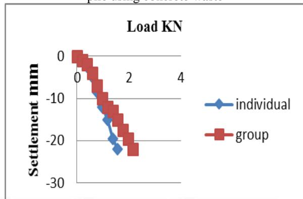
Fig. 4: comparison of load settlement behavior of granular pile using tile waste
