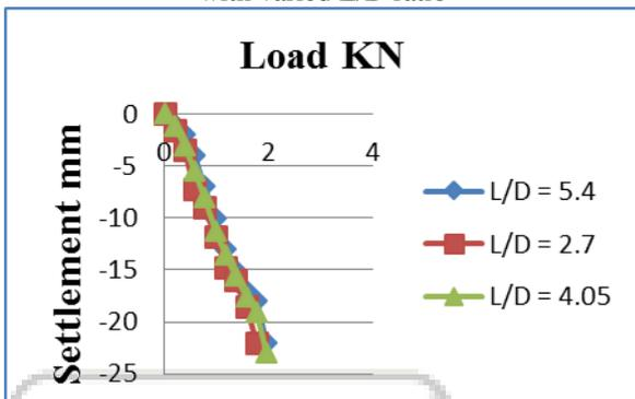
Fig. 7: comparison of granular pile formed using Concrete waste with varied L/D ratio
