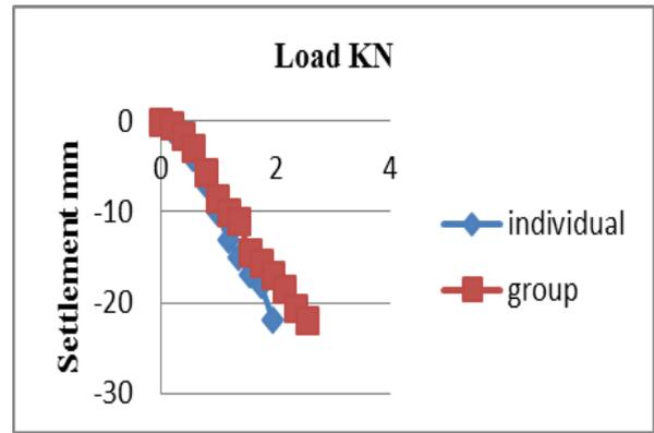
Fig. 3: comparison of load settlement behavior of granular pile using concrete waste
