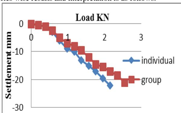
Fig. 2: comparison of load settlement behavior of granular pile using aggregates
