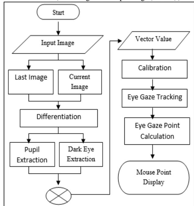
Fig. 2: The flow of the eye gaze tracking algorithm
