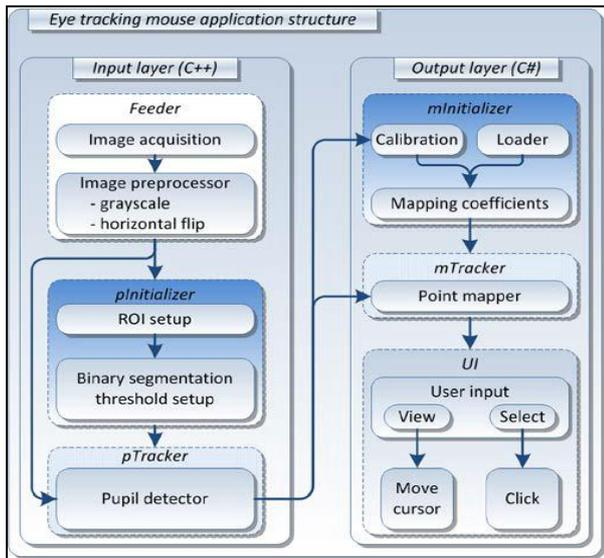
Fig. 3: Eye-tracking mouse software application
