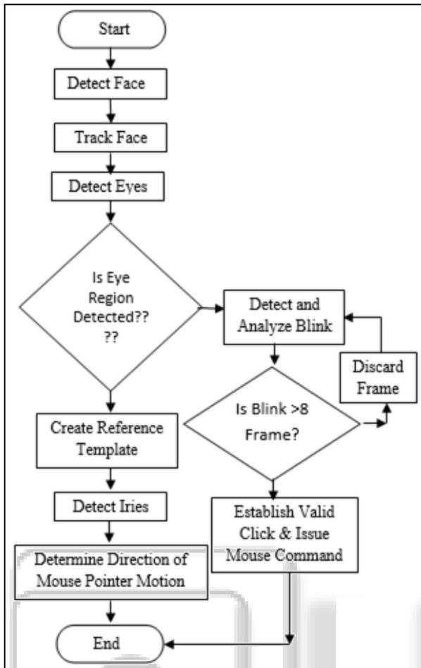
Fig. 4: Flowchart of implemented algorithm.
