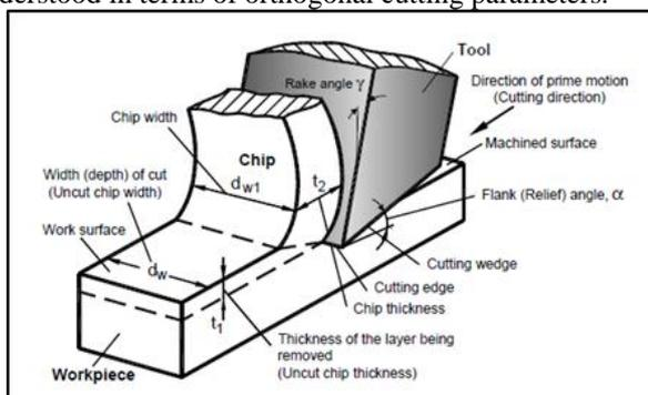
Fig. 1: Visualization of basic terms in orthogonal cutting
