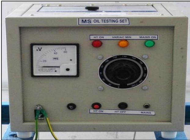
Fig. 2: Transformer Oil Test Kit
