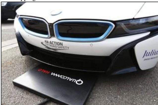
Fig. 4: Recardo using Qualcomm's wireless electronic vehicle charging technology (WVEC).
