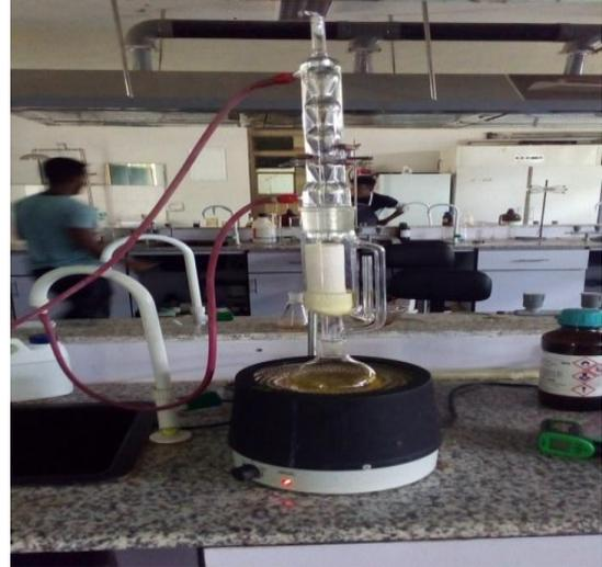
Fig. 6: Extraction of oil using soxhlet equipment
