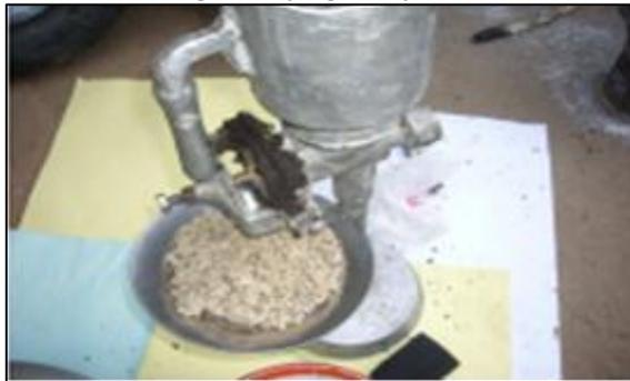
Fig. 5: Grinding the seed crystals
