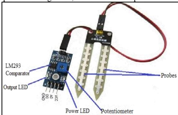
Fig. 3: The Soil Moisture Sensor
