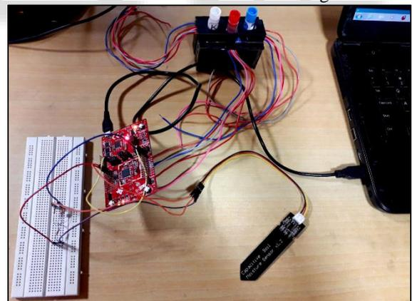
Fig. 9: The soil monitoring system
