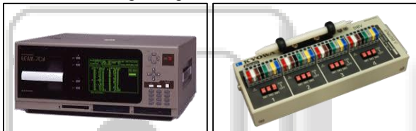
Fig. 3: Data logger and bridge box
