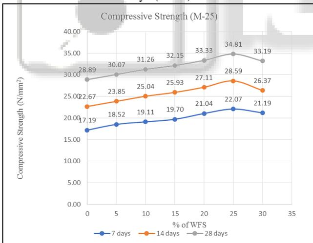
Fig. 1: Compressive Strength of cubes for 7, 14 and 28 days (M-25)
