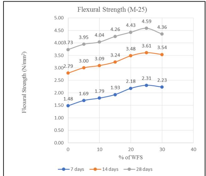
Fig. 2: Flexural Strength of Beams for 7, 14 and 28 days (M-25)
